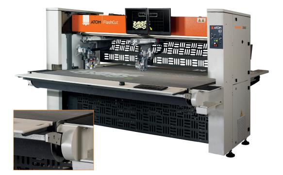
The wide cutting surface allows to process both half and full hides. The front tilting table increases the support and nesting area. Perfect for footwear and leather goods industry, it assures maximum productivity and great efficiency.
